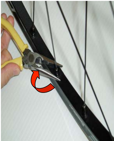
REMOVE LOCKRING WITH PLIERS NOTE LOOSENING ROTATION IS CLOCKWISE!
