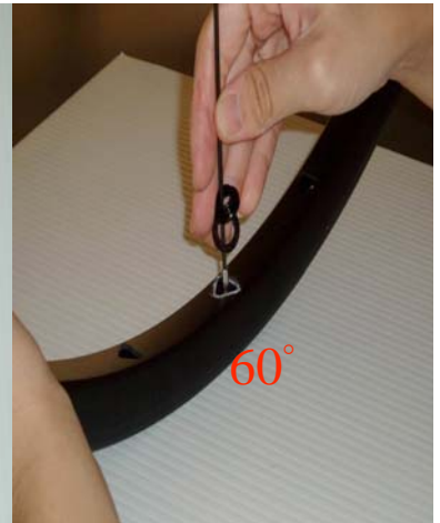
INSERT NIPPLE SEAT WITH RIM AND TURN NIPPLE SEAT 60° UNTIL ENGAGED
