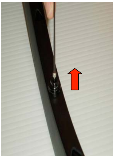
PULL ON SPOKE GENTLY TO KEEP NIPPLE SEAT ENGAGED WITH THE RIM
