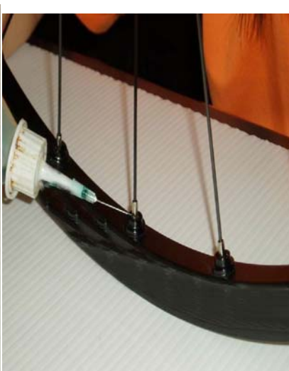
(OPTION) INJECT GREEN LOCTITE BETWEEN LOCKRING AND NIPPLE
