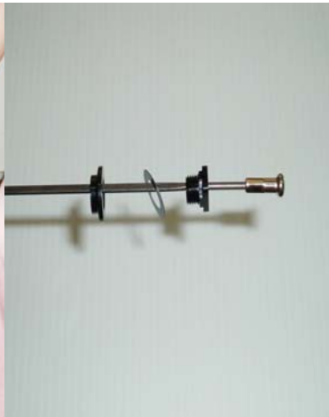
ASSEMBLE SPOKE + NEW NIPPLE + NIPPLE SEAT + WASHER + LOCKRING AS SHOWN
